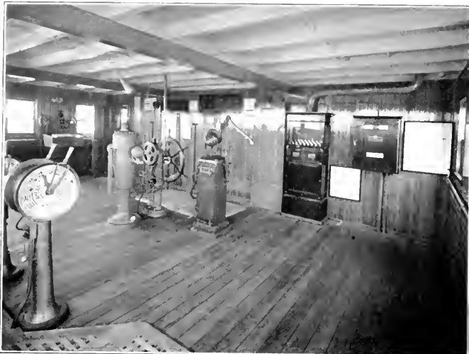
The enclosed bridge on the Steamship President Hoover featuring magnetic compass, steering stand, Sperry gyro-repeater and gyro-pilot, Rich smoke-detection cabinet, watertight door control, and engine room telegraph.
